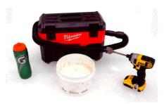
1. The tools we use are a battery-operated wet vac (or I use a large turkey baster), water bottle with warm water, cordless drill with a 1½ spade bit and a clean bucket. Some facilities have had success with hole saws or even flattening the tip on a spade bit to get deeper into their marsh peg sleeve or tube. 1½ inch spade bit used to clean out the marsh peg sleeve in the floor.
