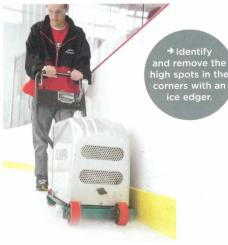
Identifying these areas is very important for several reasons. First, once the IR blade starts shaving into the white ice paint it will start to dull quickly, so you will need to be prepared to change the blade frequently from this point forward. Secondly, as you shave through the paint and the IR blade hits an area of frozen sand it will render the blade unusable, and the blade will need to be replaced
